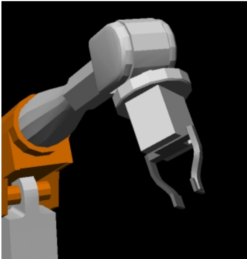
Figure A3 Interactive GUI process simulation: The gripper of the revolute Robots of Fig. 2. Created by Richard Silva with Visual Nastran.
