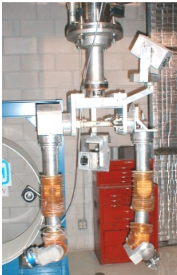
Figure 2. Dual slave arm end effector in the UNLV Robotic Hot Cell Unit. The master is configured identically, and is guided by a human operator.
