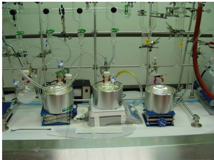
A depiction of the Schlenk line experimental set-up for the generation and storage of liquid ammonia, solvent transfer for the dissolution of iodine, and the cannula transfer of solution for reaction with uranium.
