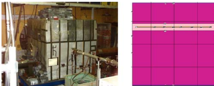
RPI's LSDS (left), and a cross section at x = -37.5\text{cm} showing the assay channel and fuel pin (the x axis is positive along the beam line).
