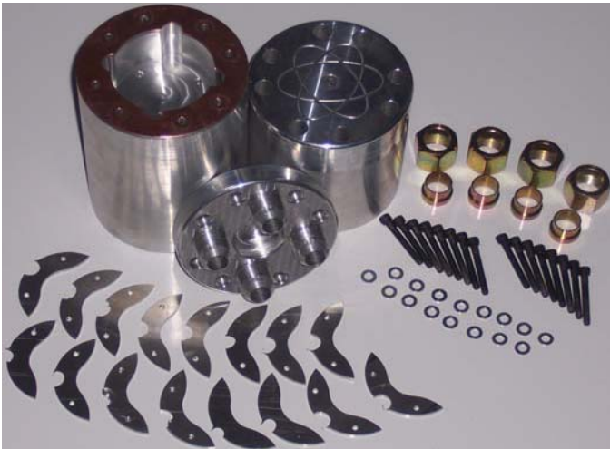
Components of the CETON (Cooled Electron Target — Optimized for Neutron production) excluding tungsten-copper disks for converting electrons to photons. The W-Cu disks fit in the cavity at the upper left. In addition, the body is bored to accept a 10" aluminum-clad uranium photo-neutron generator.
