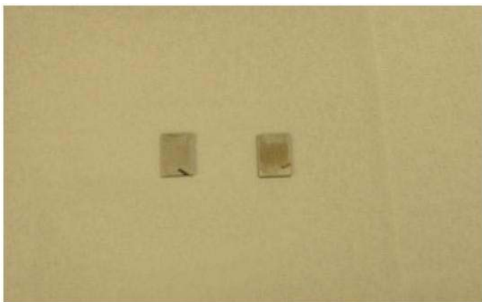
Photograph of two anodized samples showing the porous alumina on steel.
