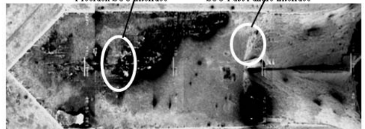
Scanning electron microscope micrographs of double-cantilever beam specimens with 0.5 wt% Si subjected to SCC testing at 100°C in acidic solution for 30 days.
