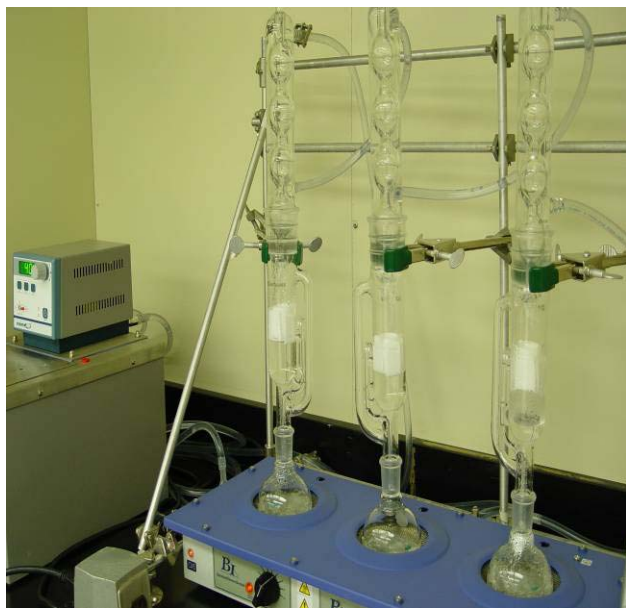
Soxhlet apparatus to compare corrosion resistance and to determine long-term behavior.
