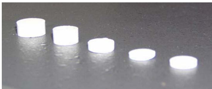
MgO-ZrO 2 pellets synthesized from precipitation of metal salts.
