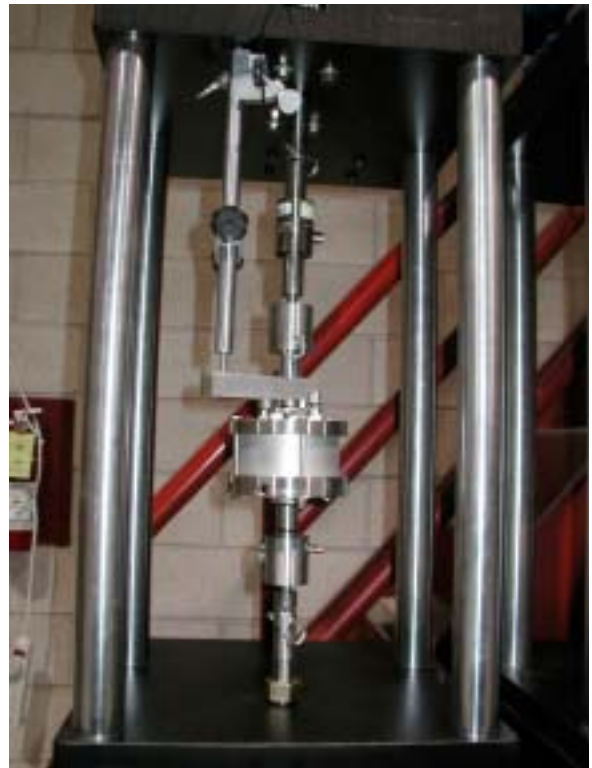
Tensile testing machine with elevated temperature jacket.
