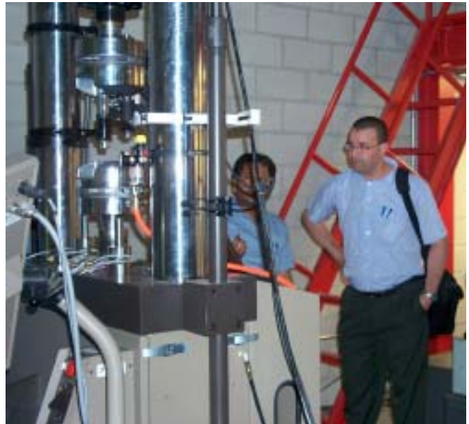
Heavy duty torsion and tensile testing machine.
