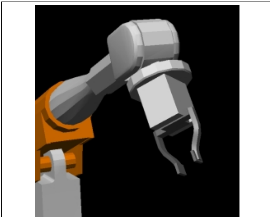
Figure A3 Interactive GUI process simulation: The gripper of the revolute Robots of Fig. A2. Created by Richard Silva with Visual Nastran.
