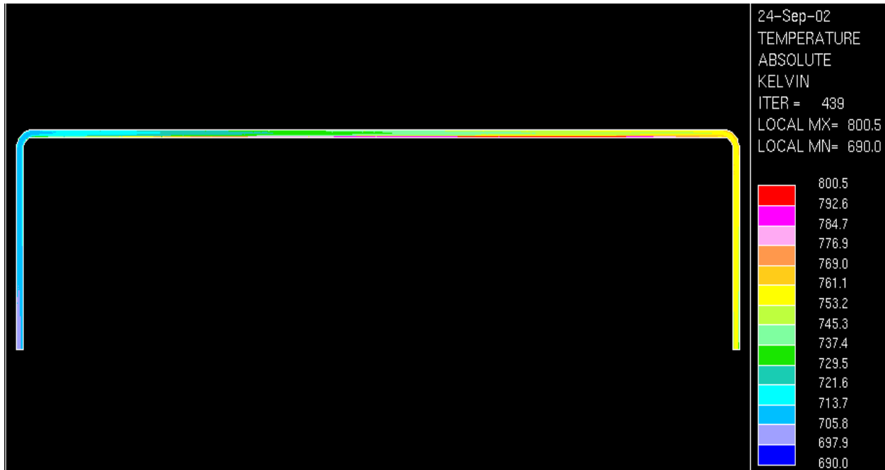
Fig -44: Fluid Temperature for Loop2 at an Axial Plane of the Pipe
