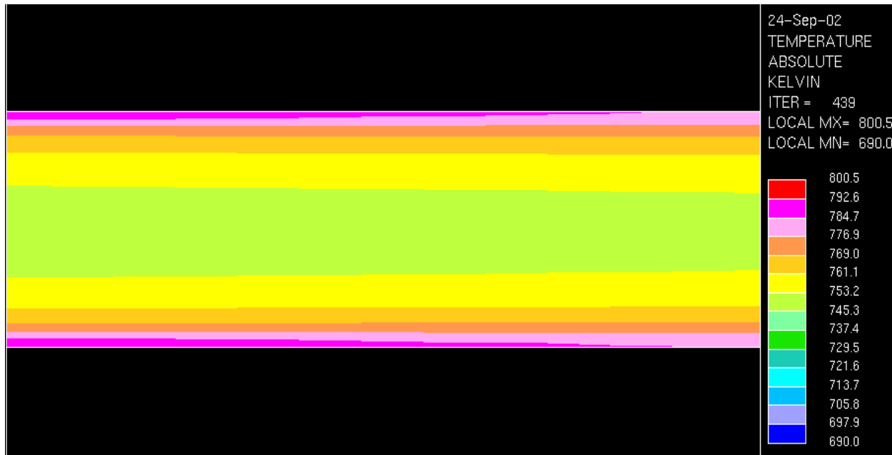
Fig -47: Fluid Temperature at the Cooling Zone in the Loop2
