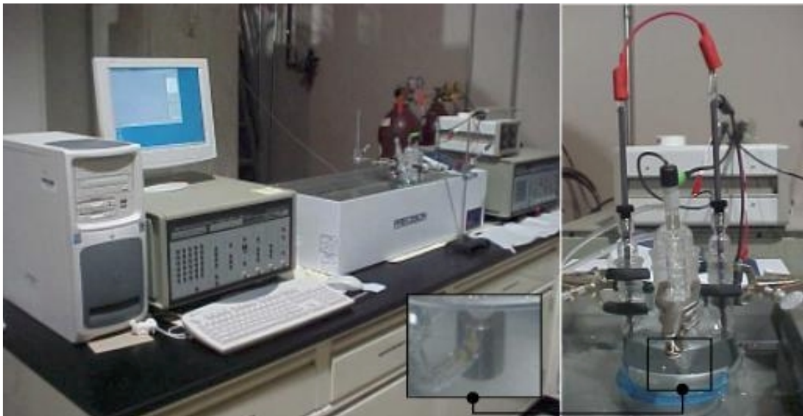
Figure 2. Electrochemical Polarization Test Setup
