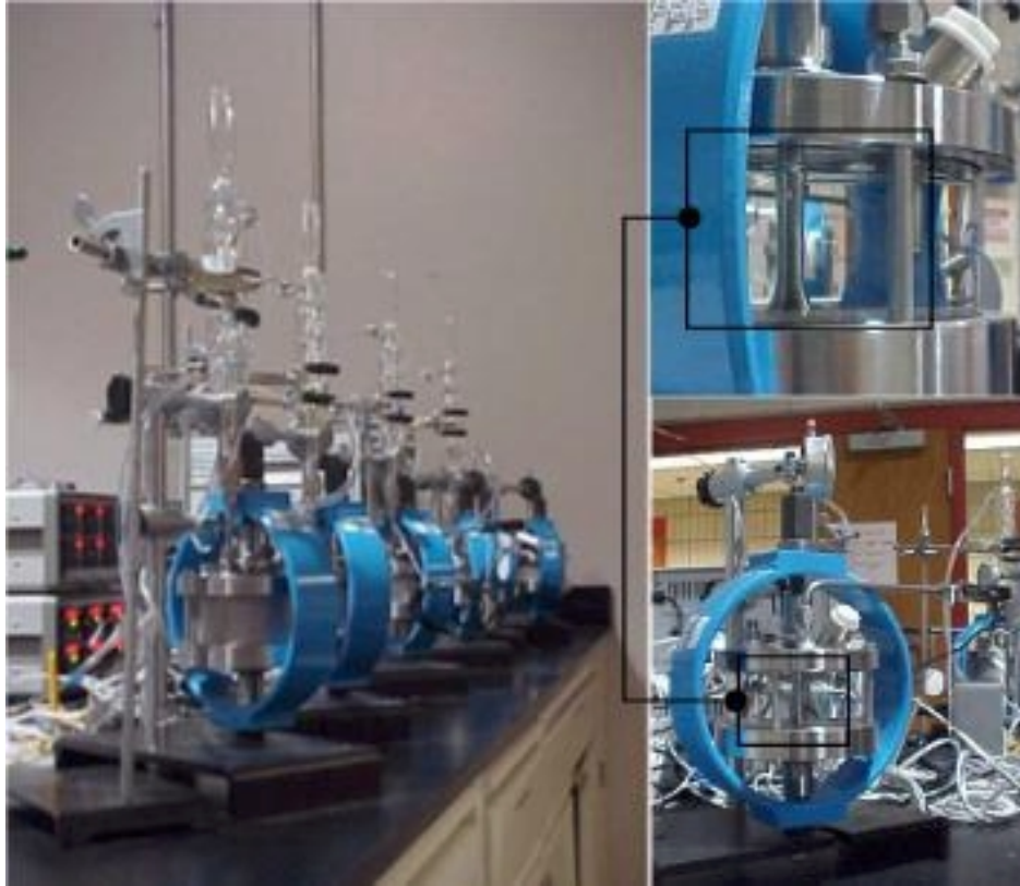
Figure 1. Constant-Load SCC Test Setup
